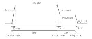
**Note:** If the pre-programmed schedule above is followed, the lights will reach the brightness set for daylight at 9:15 AM and will be completely off at 8:15 PM.
